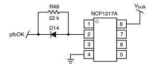
Figure 12. Enabling / Disabling the Downstream Converter
