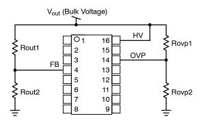
Figure 8. Configuration with Two Separate Feed-back Networks
