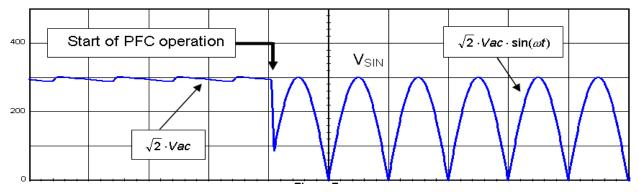
Figure 4. Typical Input Voltage of a PFC Stage
